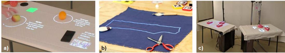
*We presented three different prototypes of interactive tabletops with projected augmentations in the exhibition: a) first prototype: illustrating object recognition and projection of informational content; b) second prototype: projecting of cutting patterns onto fabric, adjustable by manipulating a paper proxy with optical markers; c) third prototype: two separate tables virtually linked and objects dynamically mirrored onto each other.*
